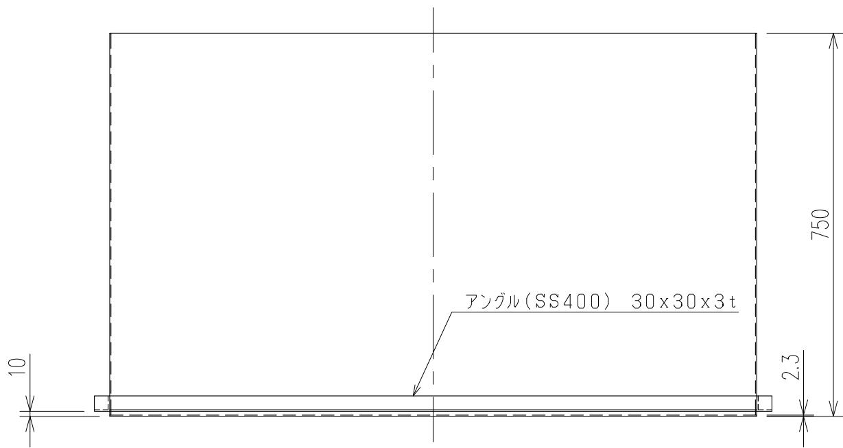
材質: SPHC  $t = 2.3\text{ mm}$
